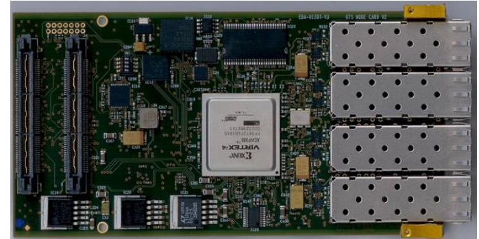
GTS V3 mezzanine with Virtex 4 (Padova design for AGATA)
